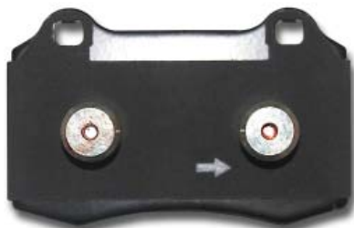
The arrows should follow the direction of disc rotation.
