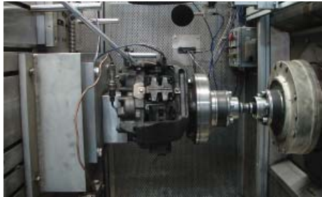
Brake assembly unit being tested inside a sound booth.
